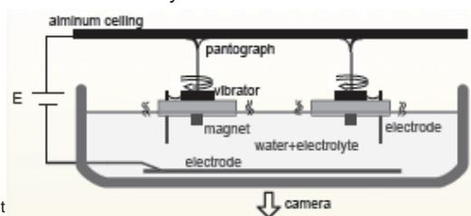
The vibrating modules are powered using a pantograph system and can move using vibrating motors.
