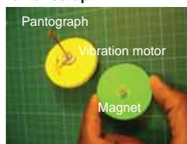
All the modules are equipped with a magnet aligned in a way such that they repel each other (north is always pointing up). The yellow module has a vibration motor (vibrating module) and the green module doesn't (passive module).
