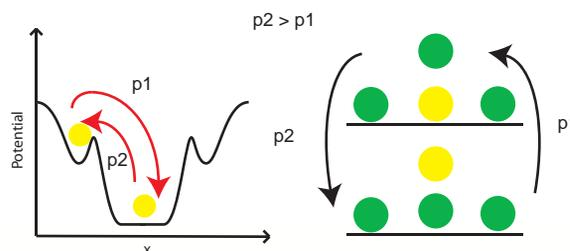
If there was a potential well surrounding the yellow modules, we would also observe assembly in the center. The yellow modules are therefore subject to a potential well-like interaction created by the presence of the green modules. The self-sorting behavior can also be explained by the fact that, the probability  $p_2$  that the vibrating yellow modules move from the corners of the water tank to the middle is higher than the probability  $p_1$  that they move in the opposite direction.
