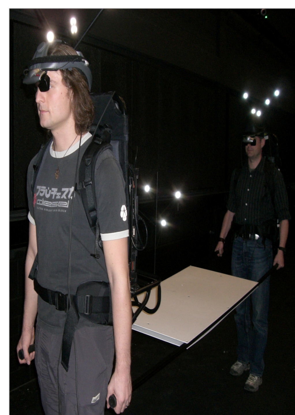
Method: Two participants carry a stretcher through a large room. Both participants head movements and the stretcher are tracked using an optical tracking system. In the HMD they see the virtual world and a representation of each other.
