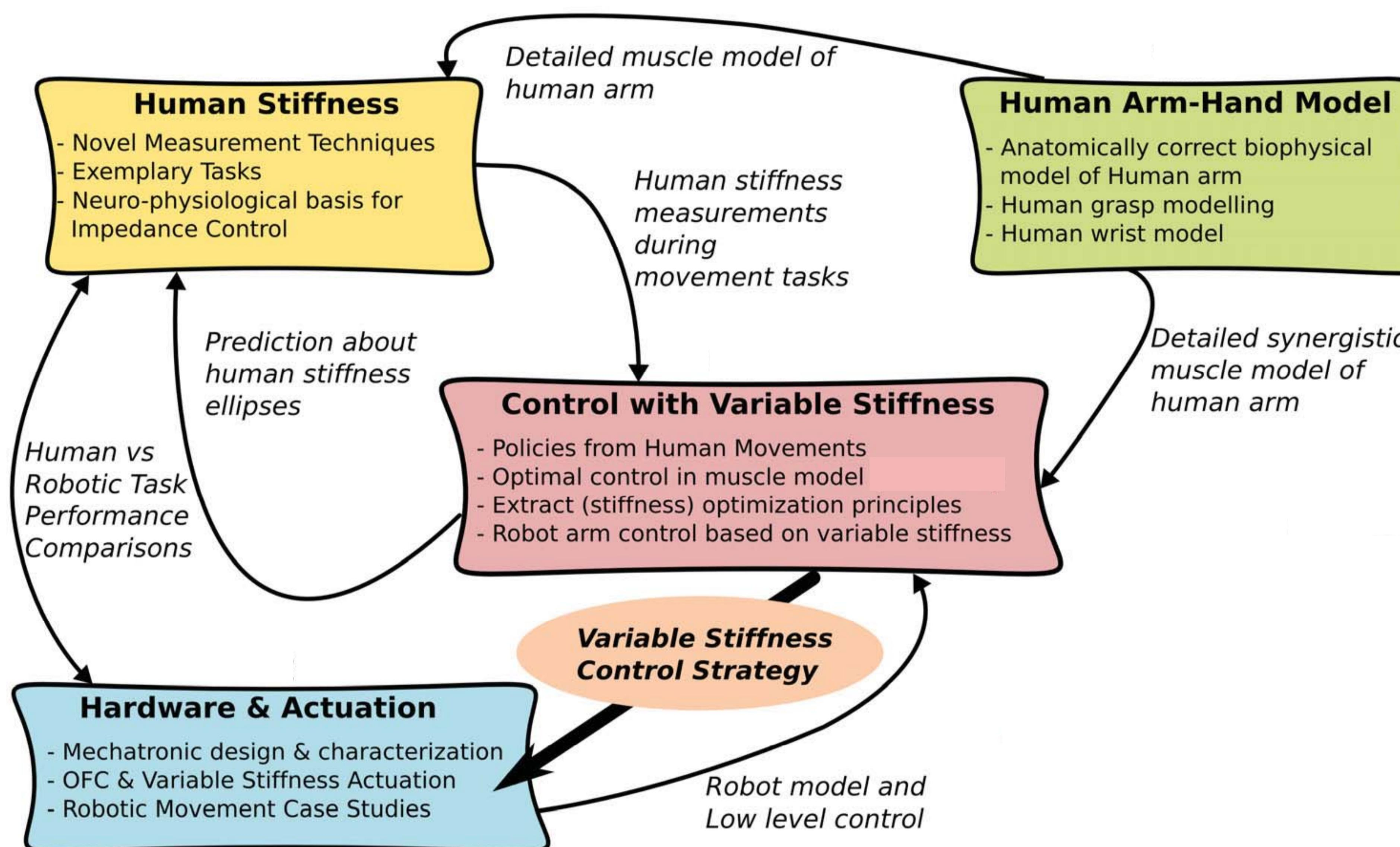
We investigate the stiffness of the human arm and hand (i.e., grasp force) involving detailed skeletomuscular models thereof, to serve as a basis for the development and control of a highly biomimetic robotic hand-arm system. A detailed skeletomuscular model of the human arm and hand is developed based on a deep biological understanding and used as an interface. Cost functions for motor actuation are learned from the results of the human stiffness experiments and used for an optimal controller.
