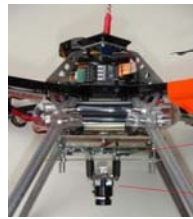
Figure 2. Gumstix and camera setup
