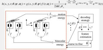
**Disparity and optic flow estimation** (real-world situation) The images are acquired by moving stereo cameras, thus both ego-motion and independent motion of other objects in
