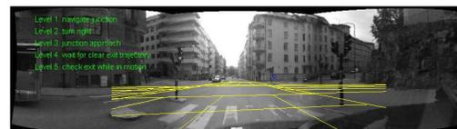
FIGURE 5: Decision tree output projected onto the screen frame along with eye-gaze (blue dot) and junction topology/lane structure.
